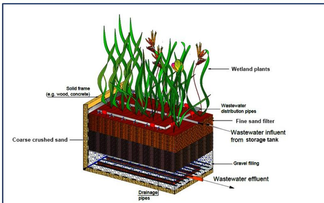
Figure 2.13. Horizontal flow constructed wasteland design.
