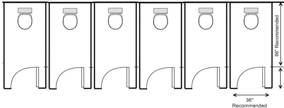
Figure 2.5 Floor Plan of the Centralized Toilet Room with Six Cubicles
