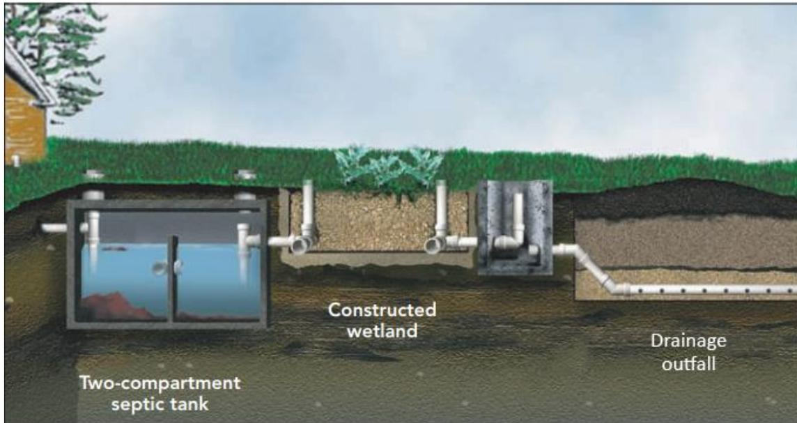
Figure 2.12 Constructed Wetland System
