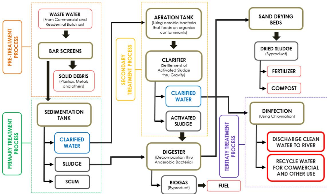
Figure 2.21. Detailed Plant Operation Process
