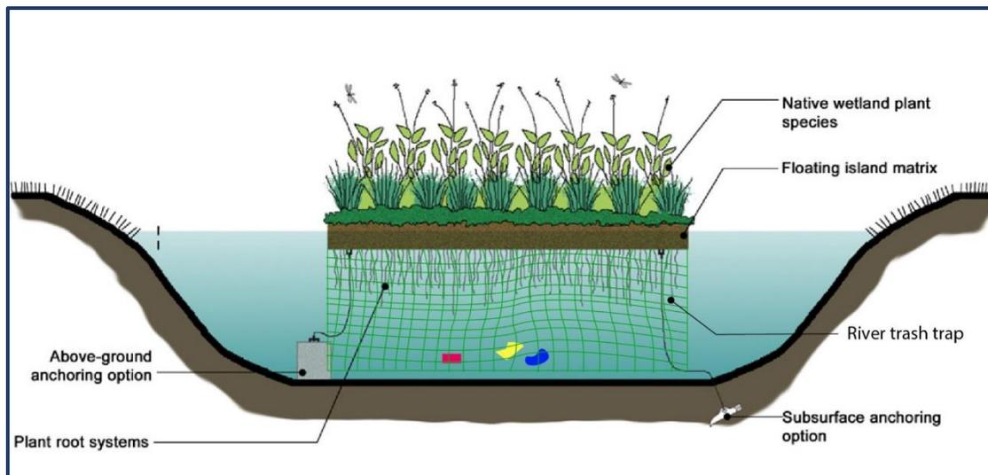
*Figure 2.17. Schematic diagram of constructed floating wetland adopted from Tanner, C. et. al. (2011)*
