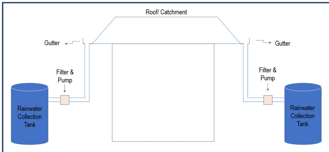
Figure 2.6 Schematic Diagram of Rainwater Harvesting System
