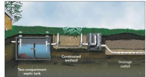
Figure 2.7 Constructed Wetland System
