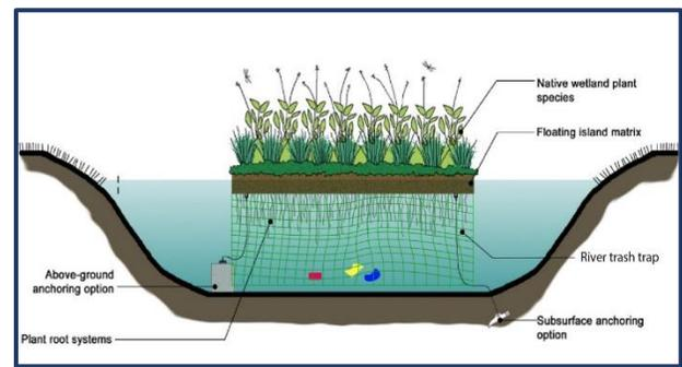
Figure 2.9. Schematic diagram of constructed floating wetland adopted from Tanner, C. et. al. (2011)
