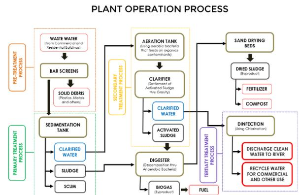
Figure 2.21. Detailed Plant Operation Process
