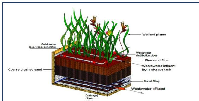
Figure 2.8. Horizontal flow constructed wetland design. Adopted from Napaldet, J. & Buot, I. (2019).
