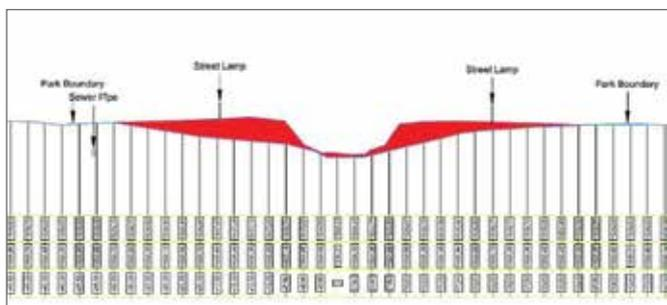
**Figure 1: Sample cross section of the canal area – the red shading shows the extent of the bulk excavation to increase conveyance**
