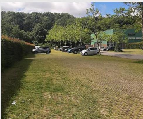
Figure 1 Car park with open grid pavement.
