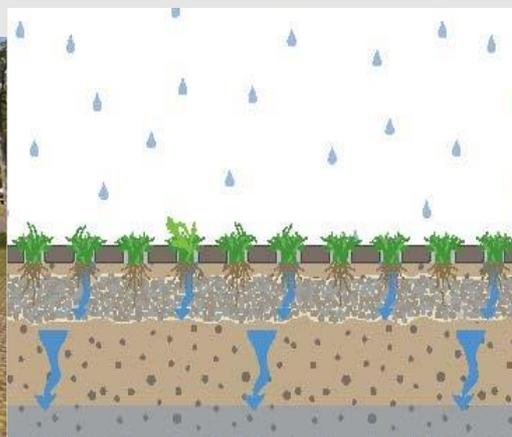
Figure 2 Water infiltration through open grid pavement. (Kenniskbank Groenblauw)
