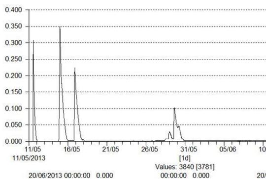
Figure 7 Water level within rain garden void following 5 rainfall events in June 2013
