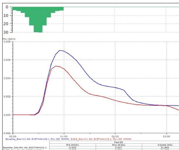
Figure 8 Model output showing reduced peak in sewer flow (in red)
